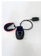
To charge the HC, first, connect the USB A wireless charger connector to the provided DC power supply and plug it into a wall outlet.
